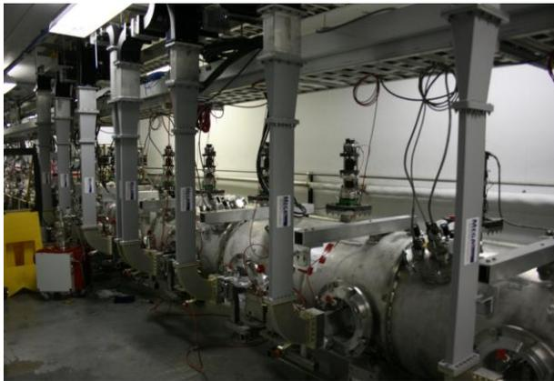
Fig. 3. New Cryomodule C-100 with Waveguide installed in South Linac
