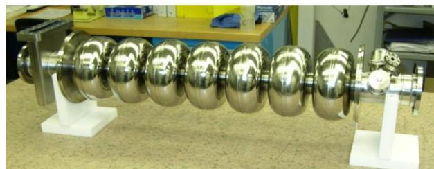
Fig. 2. Cavity of new Cryomodule C-100
