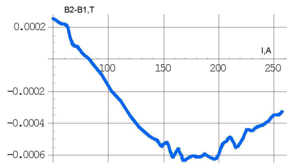
Fig. 13. Dependence of magnetic field difference in the first and second "NESTOR" injection channel dipole magnets on magnet excitation current
