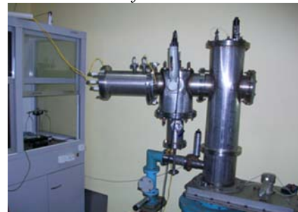
Fig. 5. Neutralizer testing device with small ion beam accelerator
