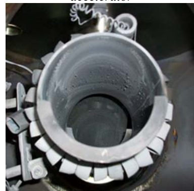
Fig. 6. Oxidized sodium vapor stream pattern on the cooler surface during approximately 1 hour air exposition after vacuum chamber opening
