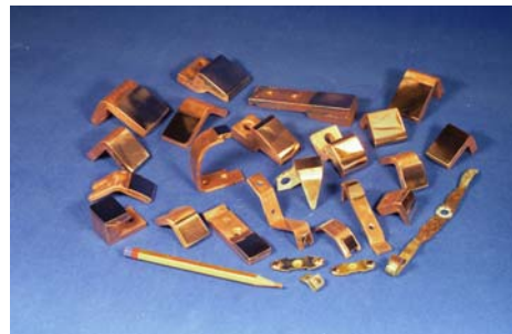
Fig. 5. General view of the sliding contact made of composition Cu—Zr—Y—Mo.
