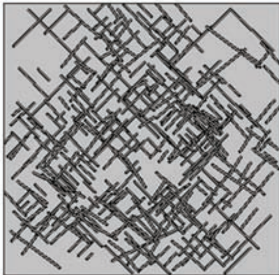
Fig. 4. Lineaments distribution with azimuth 45 and 135°.
