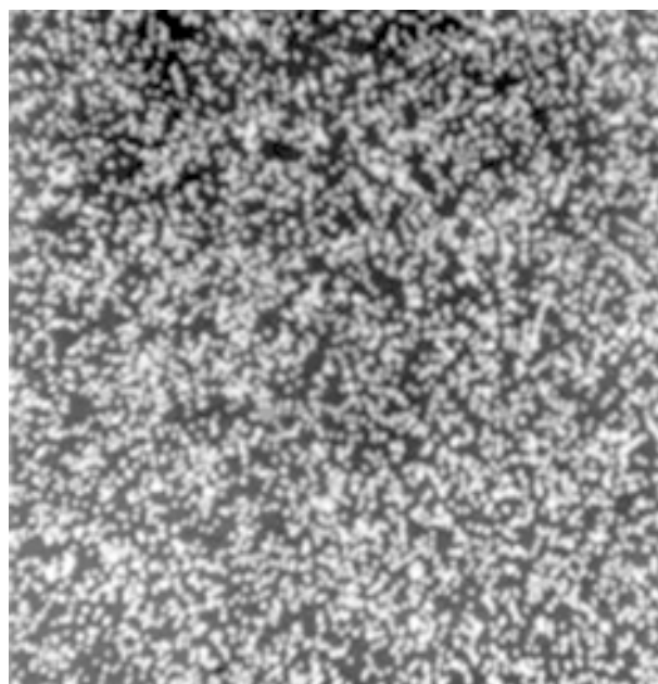
Fig. 4. The image of distribution of S atoms on a surface of TbS films in secondary X-rays ( \times 400 ).
