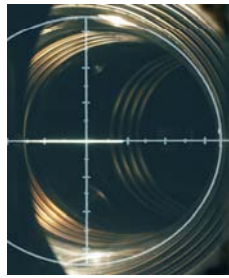
Fig. 2. Photography of a scanning rod and internal wall of the toroidal vacuum chamber in the measurement cross-section, executed through a glass window of the tangential port
