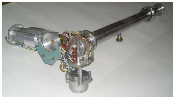
Fig. 3. The movement device of a luminescent rod
