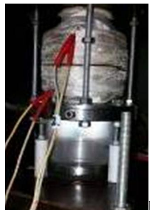
Fig. 1. Scheme (a) and photo (b) of PLS for hybrid plasma-catalytic reforming of ethanol aerosol
