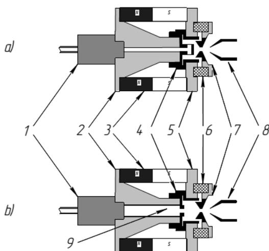
Fig. 3. Schemes of the two versions of  $H^-$  ion source: a – Source with magnetron discharge; b – source with additional hollow cathode discharge
