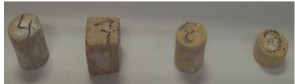
Fig.3. The samples on basis Ceramicrete for conditioning of radioactive waste
