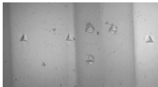
Fig. 2. First indent series with 500 nm penetration depth. The lighter surface displays the non irradiated part and the darker one the irradiated part of the sample
