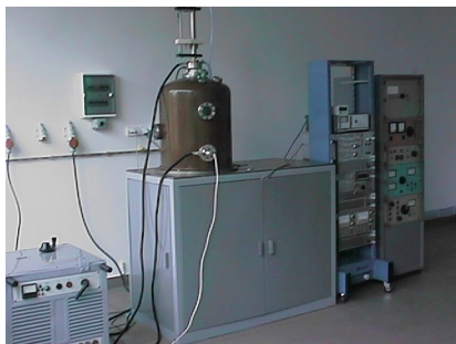
Fig.10. New UHV stand with cylindrical Nb-cathode.
