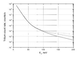
Fig.4. Energy dependence of tritium count rate for different He<sup>+</sup> density profiles. NPA collimator: wS=1.3.e-4 cm2 strd, energy resolution  $\Delta$ E=0.1 E, Detection Efficiency K(E) = 0.05 – 0.9 in presented energy range. Solid line – without He<sup>+</sup>; dashed line – corona (n<sub>He+</sub> = 1.6·10<sup>5</sup> cm<sup>-3</sup>); dotted line – n<sub>He+</sub> = 6·10<sup>5</sup> cm<sup>-3</sup>
