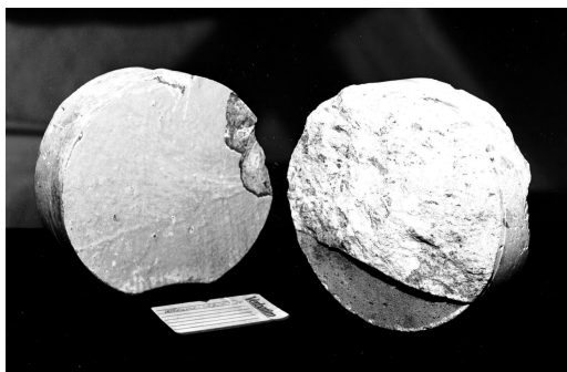
Fig. 1. Concrete cores (pristine state, K1 from the left)
