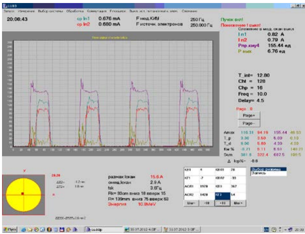
Fig. 6. The display screen on an operator's console of the LU-10 accelerator
