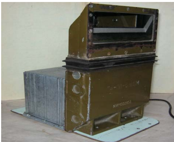
Fig. 3. Camera video observation, which used in the electron accelerator bunker, enclosed in the protective lead housing
