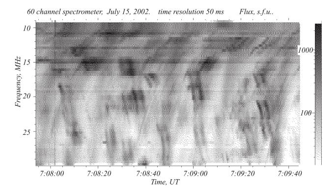
Figure 5. Fragment of the "drift pair" storm on July 15, 2002
