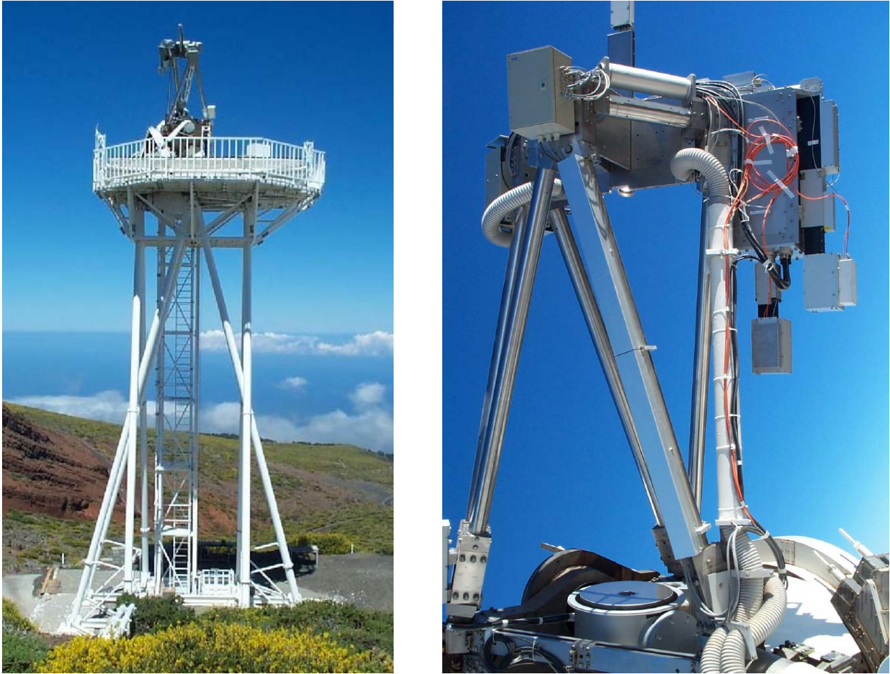
Figure 7. The Dutch Open Telescope at the Spanish Observatorio del Roque de los Muchachos of the Instituto de Astrofísica de Canarias on La Palma. Left: 15-m high open tower with telescope. North is to the right. The triangular geometry of the tower stilts is such that the platform can only move laterally, without tilt, so that the telescope (focused at infinity) shows no image motion even in strong wind buffeting. Right: close-up of the telescope. The mirror diameter is 45 cm but the mount can accommodate a 140 cm mirror. The flexible tubes serve for air suction around prime focus. The reflective heat stop is water-cooled. The boxes at the top contain the multi-wavelength imaging system with six CCD cameras and a phase-diverse focus monitor. Glass fiber links to the Swedish telescope building housing the Swedish 1-m Solar Telescope (SST) transport both the control signals and the image streams. The new DOT Speckle Processor is placed in the nearby building housing the Carlsberg Meridian Telescope, also connected via glass fibers. The SST uses adaptive optics for wavefront restoration and is equipped with a spectrometer and will soon also furnish spectropolarimetry. Since the DOT and SST share identical seeing, co-pointing is a logical strategy to combine spectral diagnostics with wide-field imaging, and will frequently be scheduled the coming years. Photographs by R. H. Hammerschlag
