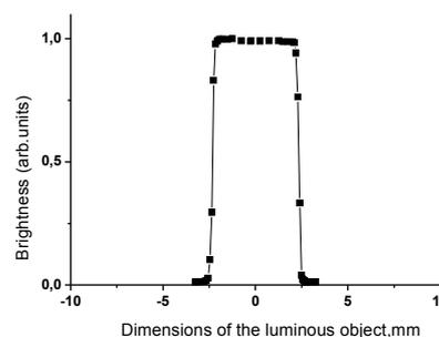
Fig. 2. Distribution of brightness of an enlarged image of the incandescent lamp ribbon at a transverse scanning with an ideal mirror (Al) in use
