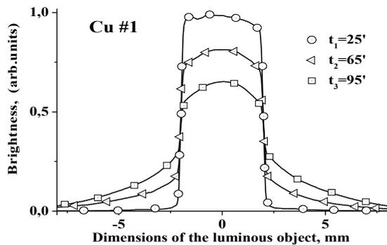
Fig. 4. The set of curves for dependences of light intensity transmitted by the small-grain Cu mirror on the linear size of the light object at successive exposures to ion bombardment. Total times of exposure are in the insert
