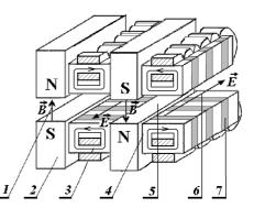
Fig. 1. Design of the stationary linearly polarized EH-cooler (only one period). There: 1 is the vector of induction of the undulative magnetic field B, 2 are the poles of permanent undulator, 3 are directions of magnetic fluxes in the ferrite cores, 4 are the inductors, which consist of the ferrite cores and winding, correspondingly, 5 is the accelerating channel, 6 are vectors of intensity of the vortex electrical field E.
