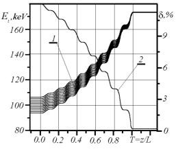
Fig. 3. Dependencies of kinetic energy for ten electrons (which differ by initial energies only - curve 1), and relative energy spread (curve 2) on the non-dimensional longitudinal coordinate T = z/Lfor the longitudinally inhomogeneous model. Here: the intensity of the electrical field is =190 kV/m, the period of undulation is 20 cm, the system length is 1 m.
