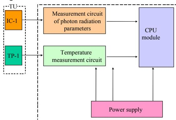
Fig. 4. Block-diagram of measurement channel.
