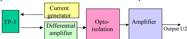
Fig. 6. Block-diagram of temperature measurement circuit.
