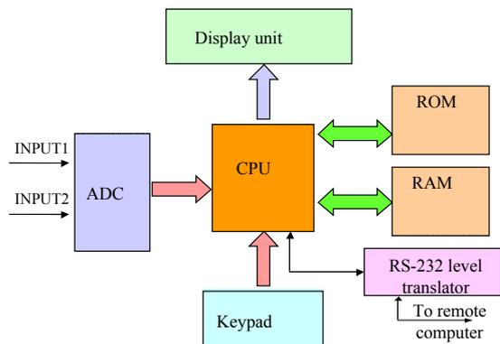
Fig. 7. Block-diagram of the CPU module.
