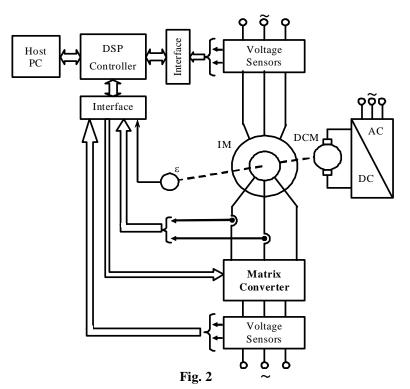
1. A 7.5 kW slip-ring induction motor supplied by a matrix converter, operating at 12.5 kHz switching frequency.
