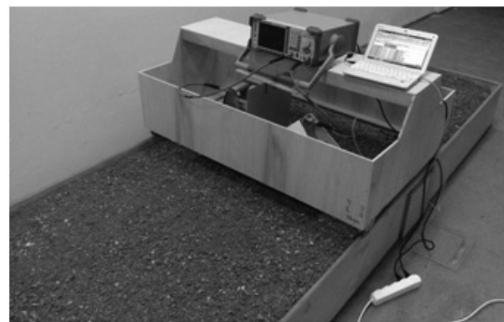
Fig. 1. Measurement set up with network analyzer
