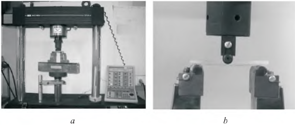
Fig. 1. Experimental setup: (a) Instron 8516 servo-hydraulic testing machine; (b) specimen under 3-point bending test.
