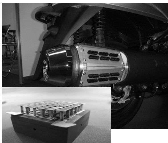
Fig. 11. Thermoelectric power generation module and system mounted on the muffler of a motorcycle.
