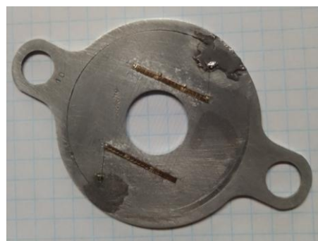
Fig. 10. Collector view, it upgraded by AlSi (1%) rod system with 25 \mu\text{m} rod diameter and distance between rods – 1 mm
