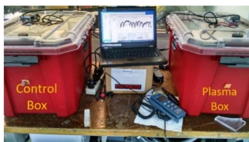
Fig. 1. Experimental stand for studying the effect of ethylene plasma-chemical oxidation on the efficiency of kiwifruit storage
