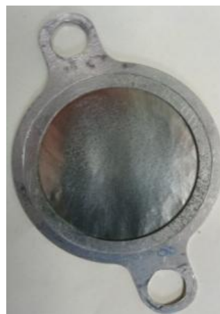
Fig. 3. Experimental target holder as a constructional element of the secondary emission monitor system
