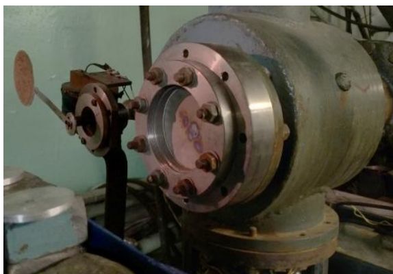
Fig. 2. The titanium foil of 50 \mu\text{m} thick after extreme experimental conditions (direct beam line during the operation of 30 MeV electron beam accelerator)
