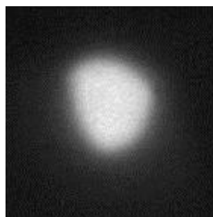
Fig. 4. Electron beam print (inverse image) on the glass plate after 15 MeV electron beam transmitted through 125 \mu\text{m} Kapton®
