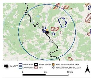
Fig. 2. A map of the 30-km zone of the Rivne Nuclear Power Plant (RNPP) with areas where karstsubsidence rocks are located
