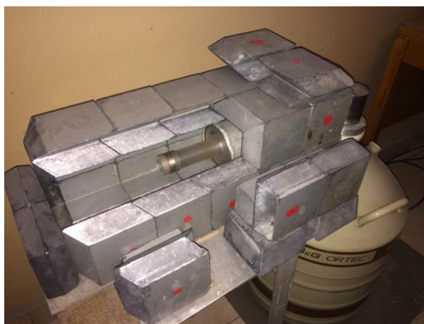
Fig. 2. Photograph of the HPGe-detector with the calibration \gamma -sources fixation
