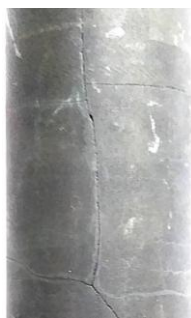
Fig. 3. Superficial cracking of CCFBPyC on Ni with ground off asbestos sheath
