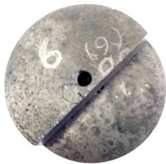
Fig. 5. External view of the CCFBPyC sections and the pancake on the border of the CCFBPyC and lower buffer
