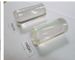
Fig. 4. The samples of ^{arch}PbWO_4 of the second crystallization
