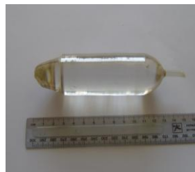
Fig. 3. Single crystal ^{arch}PbWO_4 of the first crystallization
