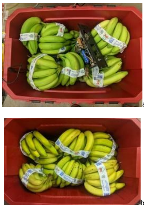
Fig. 3. Photo of bananas stored in the container, the air in which was treated by a plasma chemical system (a) and control container (b)
