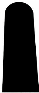
Fig. 2. Shadow electron microscopic image of a tungsten tip after high-field processing in liquid nitrogen, \times 30000
