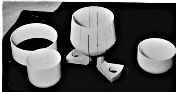
Fig. 4. Crucible and elements of the heating unit of the growth unit
