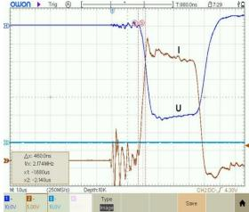
Fig. 4. Voltage (U) and current (I) pulse on the secondary winding of the pulse transformer of the technological accelerator LINAC-40: 15 A/div, 30 kV/div, 1 uS/div
