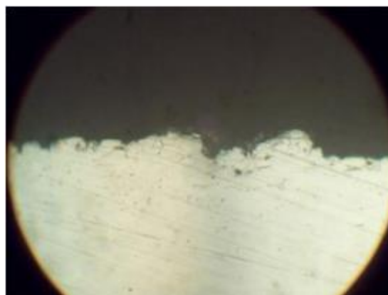
Fig. 2. Intergranular corrosion on steel samples 12X18H10T, x200
