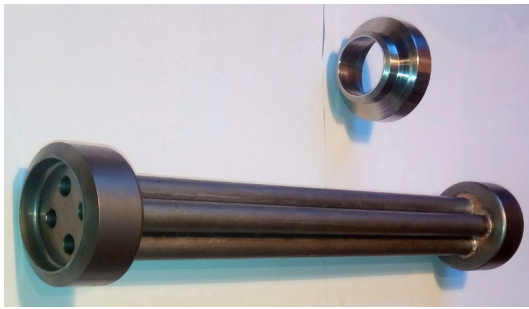
Fig. 2. Irradiation cell with flanges and mating appliance before its welding into the SCWCL assembly
