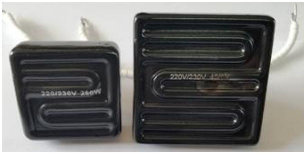
Fig. 6. Appearance of heating elements. 260 W (60×60 mm) – left, 450 W (80×80 mm) – right
