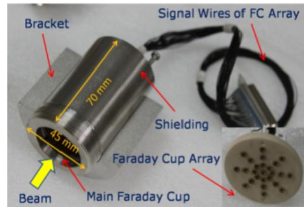
Fig. 10. Photo of the pepperpot beam distribution measuring device
