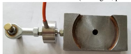
Fig. 6. Samples holder with pressure (force) tensometric gauge
