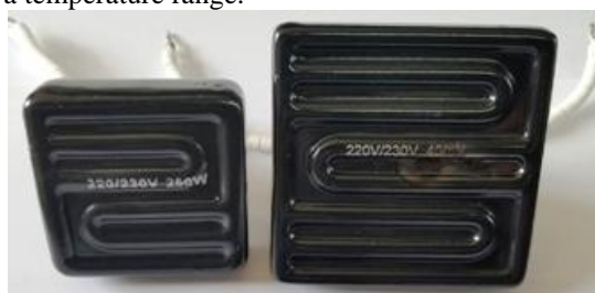
Fig. 5. Appearance of heating elements. 260 W (60×60 mm) – left, 450 W (80×80 mm) – right
