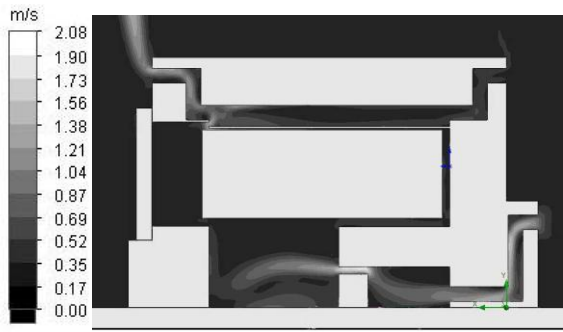
Fig. 5. Velocity contour of ventilated air inside storage module with SNF of RBMK-1000
