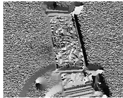
Fig. 3. The image of gradient module of the corresponding segmented thermographic image (see Fig. 2)
