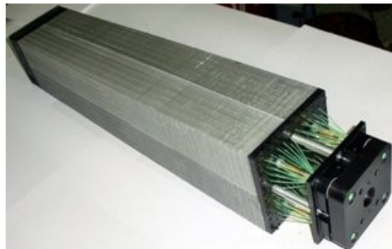
Fig. 1. Photo of a single module consisting of 4 cells with 220 layers of scintillator and absorber
