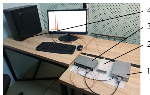
Fig. 10. Spectrometric stand: 1 – test box; 2 – ADC; 3 – amplifier-shaper and DC/DC-converter; 4 – computer
