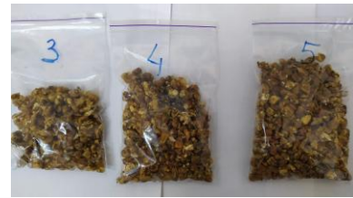
Fig. 8. Maize grain contaminated with Aspergillus flavus and treated by ozone during 3, 4, and 5 days
