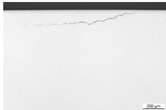
Fig. 2. Optical microscope image of the crack penetration in the metallographic cross section of L sample exposed with the plasma load of 0.1 \text{ MJ/m}^2 at T_{\text{base}} = 400^\circ\text{C}
