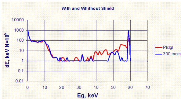
Fig.7. Scattering of E_\gamma = 60 \text{ keV} passing through a filter ( C_8H_8 ) of 10 mm – red curve
