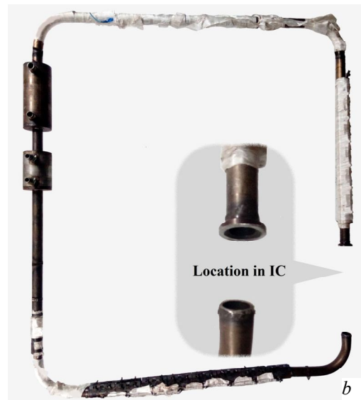
Fig. 1. Supercritical water convection loop. The scheme of the loop (a); photos inside the loop (b)
