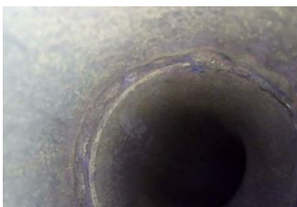
Fig. 3. The blue ring where sample № 3 is taken. A strip of rust and a nearby bluish strip are located asymmetrically along the diameter of the annular seam
