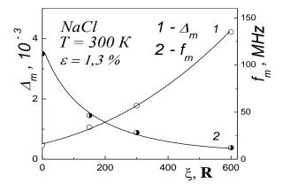
Fig. 2. Irradiation dependences of the resonance parameters  $\Delta_m$  and  $f_m$  in NaCl single crystals
