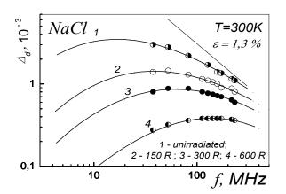
Fig. 1. Frequency spectra of the dislocation ultrasonic absorption  $\Delta_d(f)$  in NaCl single crystals with different values of X-irradiation doses
