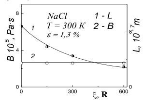
Fig. 3. Dependencies of the average effective length of the dislocation segment L(1) and the coefficient of dynamic damping of dislocations B(2) on the irradiation dose  $\xi$ . Curve 1 – the theoretical calculation of L in the framework of Stern and Granato model [29],
