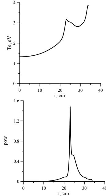
Fig. 3. Profile of electron temperature (upper chart) and power deposition profile (lower chart) in time moment  $t = 0.45 \cdot 10^{-2}$  s
